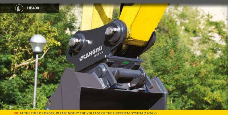
THE CR TWIN LOCK D.E. QUICK COUPLER, WITH ITS DOUBLE ACTION SYSTEM, MANAGES THE LOCKING AND UNLOCKING OPERATIONS DIRECTLY FROM THE CAB IN A FEW SECONDS. IT MEETS THE HIGHEST RELIABILITY STANDARDS THANKS TO ITS SAFETY SYSTEMS, SUCH AS THE VISUAL INDICATOR FOR THE LOCKING STATUS CONTROL, THE STANDARD BLOCK VALVE, THE DOUBLE-NOTCH PROFILE OF THE FORK. THE SIDES ARE REALIZED ENTIRELY WITH THE HB400 STEEL, GRANTING GREAT RESISTANCE.
